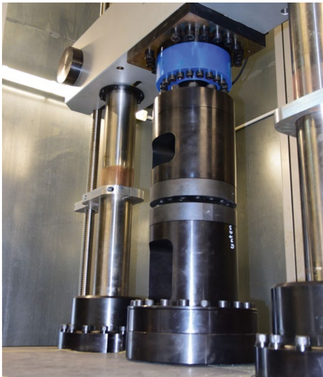
Resonance test machine for determination of a Wöhler curve
